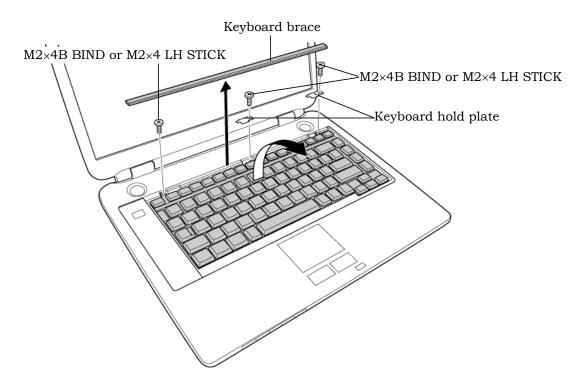
Figure 4-11 Removing the keyboard brace and keyboard hold plate
